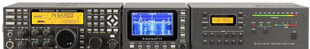
Elecraft K3 HF transceiver, P3 panadapter, and KPA500 solid-state amplifier are available in "no-soldering" kit form.
