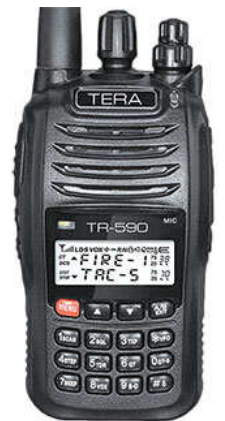
TERA TR-590 dual-band VHF/UHF 200-channel handheld commercial/amateur radio.
