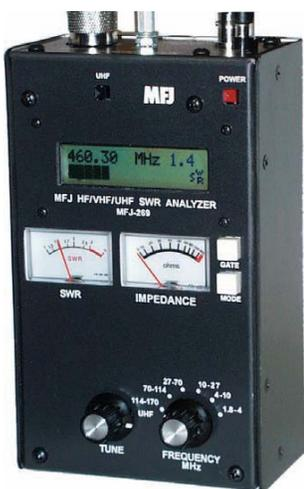
170 MHz, for \$289.95, or the MFJ-269, which adds 415 to 470 MHz to the above range, for \$389.95. It measures SWR, return loss, reflection coefficient, antenna resistance, reactance, impedance, phase angle, coax cable loss, coax cable length, distance to short or open in coax, inductance, capacitance, resonant frequency, bandwidth, Q, velocity factor, and attenuation. It has an LCD readout,
