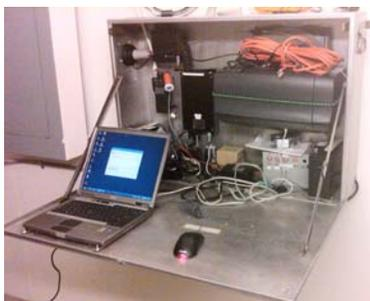
**Open ComBox showing VHF/UHF radio, TNC, laptop, and printer.**
