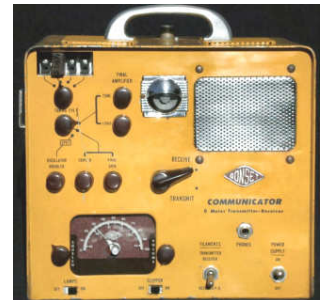
Gonset 6 Meter Communicator was a popular AM transceiver in the 1950s and 1960s.
