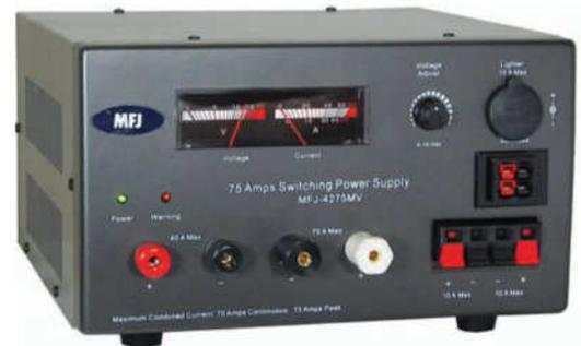
The MFJ-4275MV switching power supply delivers 75 A maximum and 70 A continuous. Input voltage is 110 Vac or 220 Vac. Load regulation is better than 1%, and ripple voltage is less than 12 mV peak-to-peak. MFJ claims that RF hash is eliminated. Front-panel output voltage is adjustable from 4.0 to 16 Vdc. Front-panel connectors include two pairs of Anderson Powerpoles, one pair of high-current five-way binding posts, a cigarette socket, and two pairs of quick connects. Weight is 10.5 pounds.
