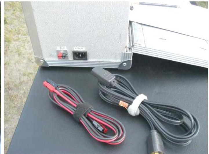
**Left side of go-kit shows DC and AC connectors and cables.**
