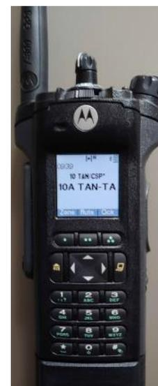
The TAN-TA simplex channel appears in Zone 10 of every 800 MHz CCCS radio, as seen in this photo of a Motorola APX portable radio.
