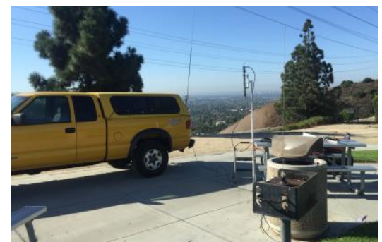
OCRACES Member Tony Scalpi, N2VAJ, set up this 2-m/70-cm/60-m portable relay station at Belmont Park, high in the hills of Orange. He beamed APRS with a Yaesu FT-1DR HT.
