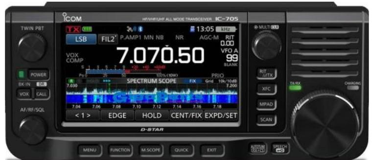
**Icom IC-705 portable SDR transceiver covers all modes on 160-10 meters plus 50, 144, and 430 MHz.**
