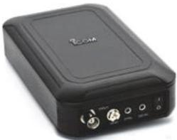
**AH-705 automatic antenna tuner covers the 1.9-50 MHz amateur bands using a long-wire element. It may be powered from alkaline batteries or external 13.8 VDC. Latching relays provide power consumption efficiency.**
