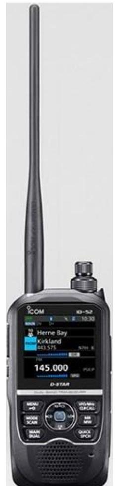
**Icom ID-52A VHF/UHF dual-band digital transceiver.**
